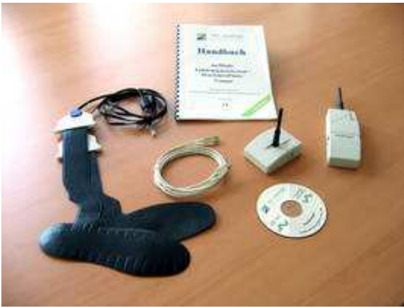
Fig. 4: Basic parts included in the MediLogic-system (source: MediLogic manual Feb. 2008)
